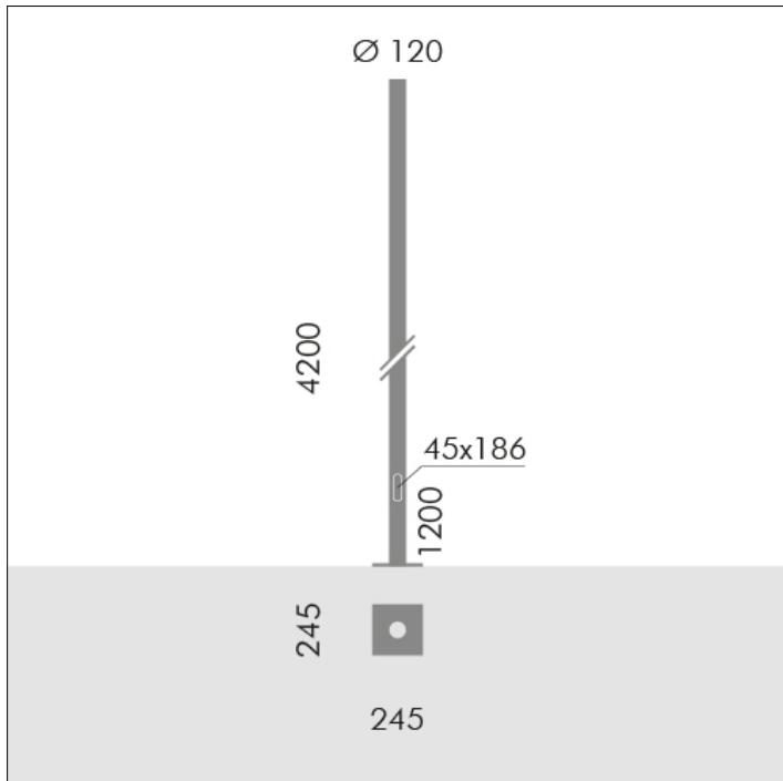
**S.2846****ZYLINDRISCHER MAST H 4,2m Ø120mm MIT
