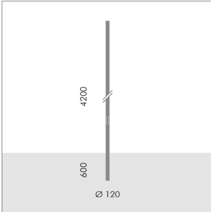
**S.2826****ZYLINDRISCHER MAST H 4,2m Ø120mm MIT ERDSTÜCK**
