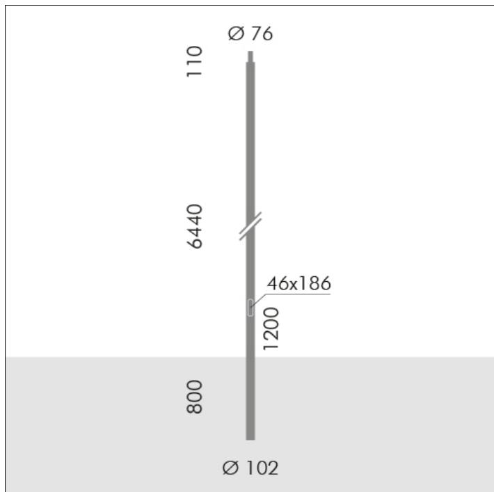
**S.2818****ZYLINDRISCHER MAST H 6,44m Ø102mm MIT
