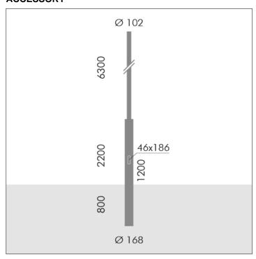
S.2817 CYLINDRICAL SHAPED POLE H 8,5m Ø 168mm -Ø102mm TO BE BURIED
