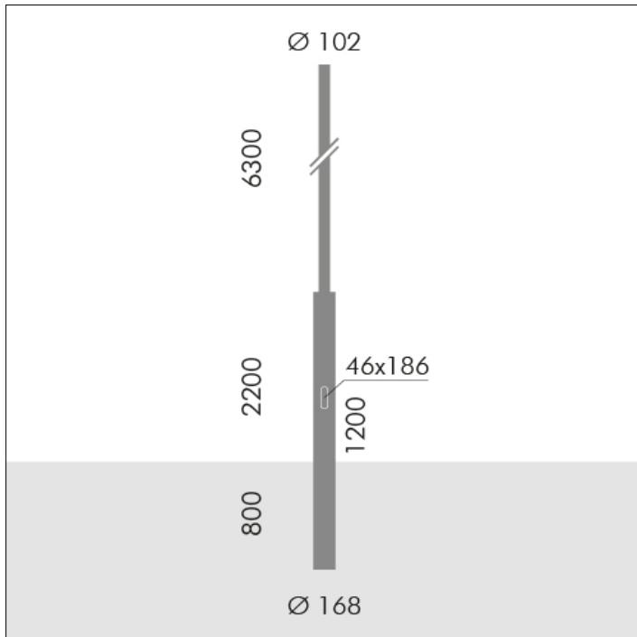
**S.2817****ZYLINDRISCHER MAST H 8,5m D 168mm- D102mm,
