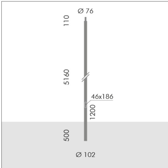
**S.2816****ZYLINDRISCHER MAST H 5,16m Ø102mm MIT ERDSTÜCK Ø76mm ZAPFEN**
