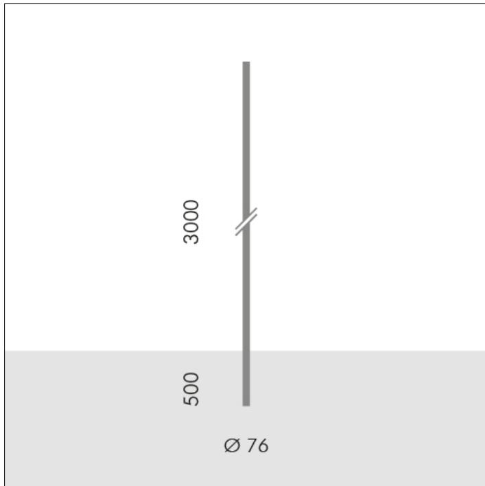
**S.2812****ZYLINDRISCHER MAST H 3,0m Ø76mm MIT ERDSTÜCK**
