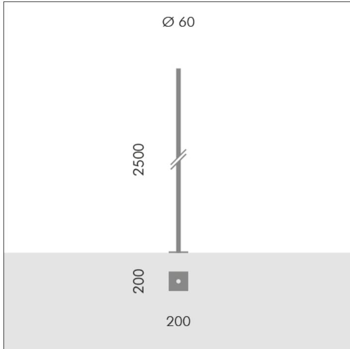
**S.2801****H 2,5m Ø60mm CYLINDRICAL POLE WITH BASE**
