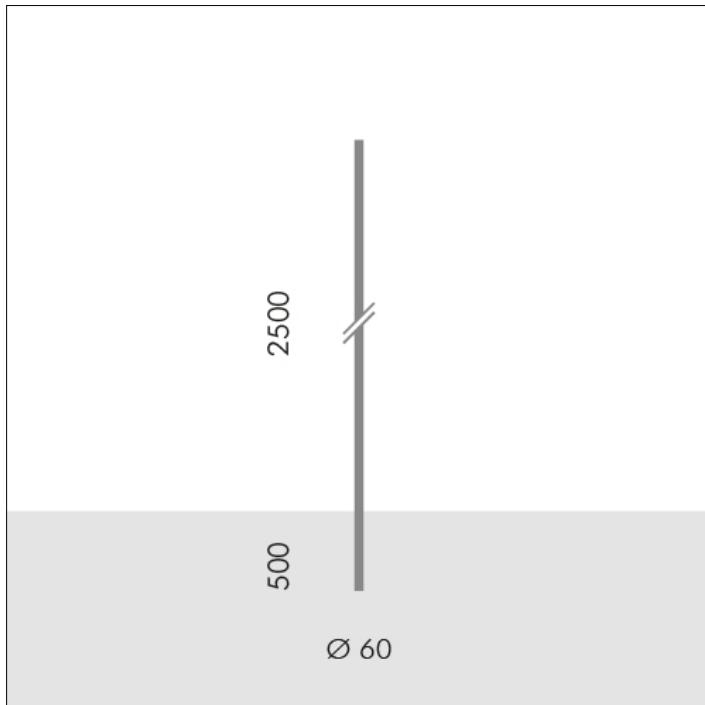
**S.2800****ZYLINDRISCHER MAST H 2,5m Ø60mm MIT ERDSTÜCK**
